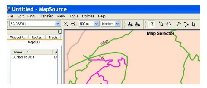
11) Hook up GPS and Click on Transfer to device. That should up load the map to the GPS.
